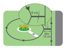
Set the Perimeter Wire CLOCKWISE around the obstacle, otherwise Robomow will drive into the Perimeter Island or won't be able to mow the area around it properly.
