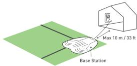
A min. of 1 meter / 3.3 feet straight wire before the base to allow smooth docking
