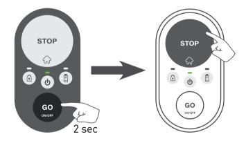
• Robomow will start driving\* towards the edge of the lawn to locate the Perimeter Wire. Once on it, Robomow will follow the wire to reach the Base Station and park there for charging.
