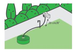
3 Drive pegs at two additional locations: at RoboRuler distance I along the edge from the first peg, and at RoboRuler distance III from the edge as shown in the picture.
