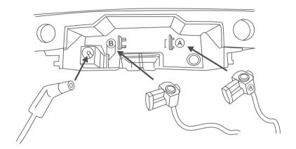
3. Note the markings for placing the Base Station Head.
