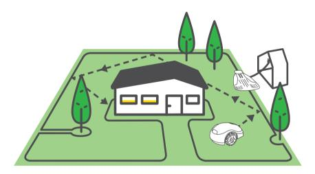
A preinstalled Perimeter Wire will set the boundaries (a "virtual wall") for your Robomow. The Perimeter Wire will be laid around the edges of your lawn and objects that you want to protect.
