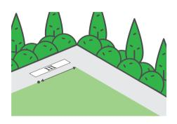
2 Pull out the wire marked A from the Perimeter Wire spool; leave a tail of approx. 20 cm / 8"; once a tail is made, put the first peg into the ground to secure this wire end.
