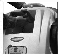
To adjust ground clearance, pull out on tab as shown and slide tab up or down.
